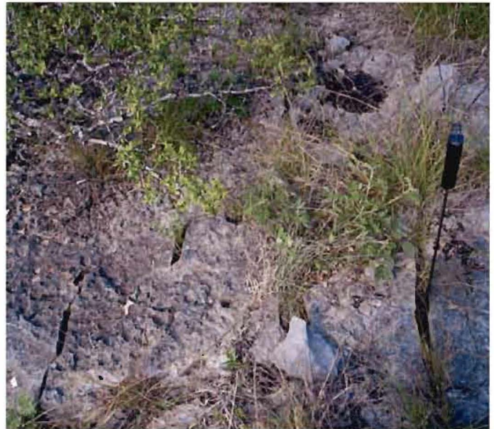
Photo #12 – Typical view of one of the few areas of solution-enlarged fractures noted throughout the Site. This photo is a view of PRF S-153.
