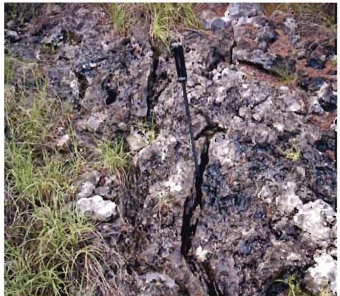
Photo #16 – View of PRF S-184 (solution-enlarged fracture).
