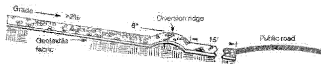
Figure 1-25 Cross-section of a Construction Entrance/Exit (NC, 1993)
