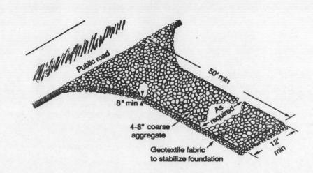
Schematic of Temporary Construction Entrance/Exit
