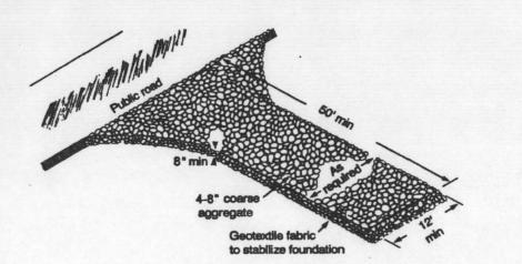
Schematic of Temporary Construction Entrance/Exit
