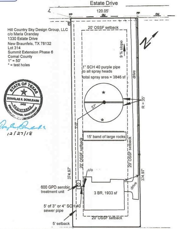
Note: water line will be sleeved with SCH 40 under drive and 10' beyond to provide equivalent protection for OSSF setback requirements of TAC 285
