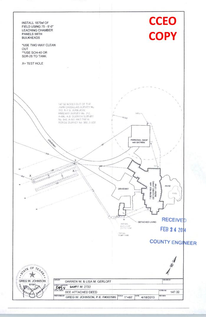
**INSTALL 1875sf OF** FIELD USING 75 - 5'-0" LEACHING CHAMBER PANELS WITH BULKHEADS
