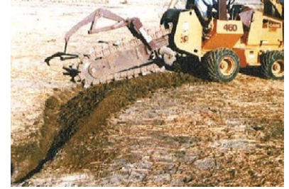
Figure 15. Trenchers make a wider excavation at turns.
