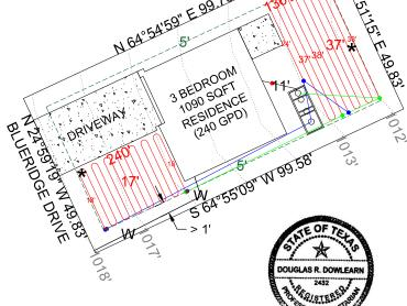
600 L.F. OF DRIP TUBING SPACED 2' APART. LINEAR FEET OF ROWS FROM HIGHEST TO LOWEST ELEVATION, RESPECTIVELY: LATERAL 1 @ 240 L.F. LATERAL 2 @ 136 L.F. LATERAL 3 @ 224 L.F.
