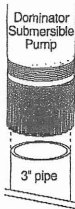
Figure 1: Insert a piece of 3" PVC pipe in the bottom of the motor to raise the pump in the tank.
