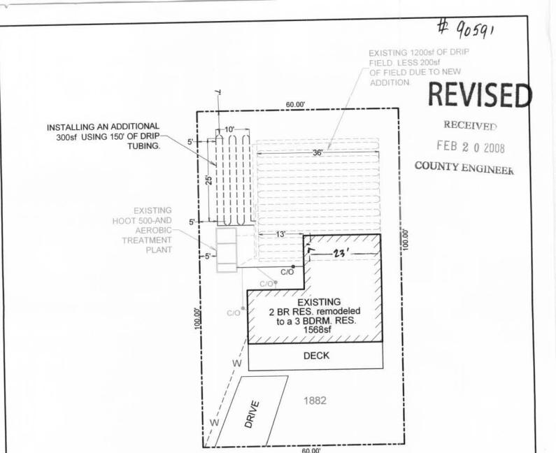
INSTALL 300sf OF FIELD USING 150' OF DRIP TUBING TO THE EXISTING 1200sf DRIP TUBING SYSTEM FOR A TOTAL OF 1300 sf. THIS WILL COMPENSATE FOR THE LOSS OF 200sf OF FIELD DUE TO NEW ADDITION (300 + 1200 = 1500 - 200 = 1300).
